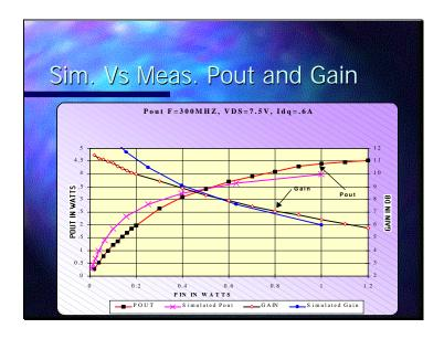
Demonstration of Accuracy in simulating Power output and gain of amplifier.
