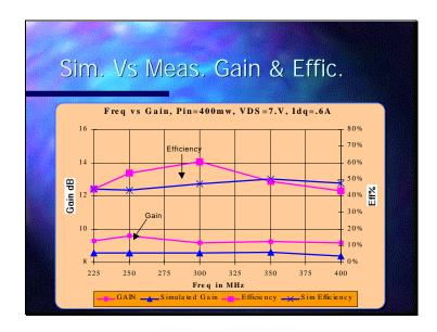
Demonstration of accuracy in simulating gain and efficiency over a broad bandwidth.
