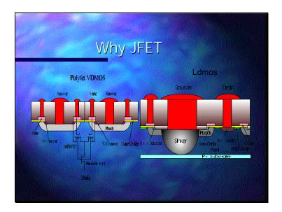
Cross section view of VDMOS showing parasitic Jfet in the vertical drain region. LDMOS has a horizontal drain drift region which is modeled by using the Jfet.
