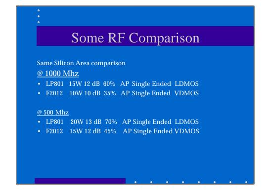
Superior Gain, Power Output and efficiency for Ldmos devices vs. Vdmos devices at high frequencies.
