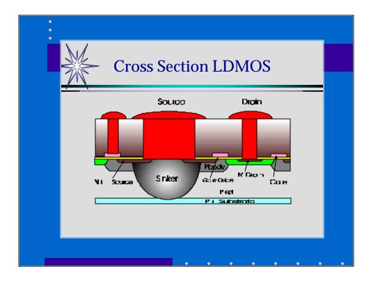
Lateral DMOS - Current flows laterally from drain to source. Bottom side of die is Source - Ground Potential
