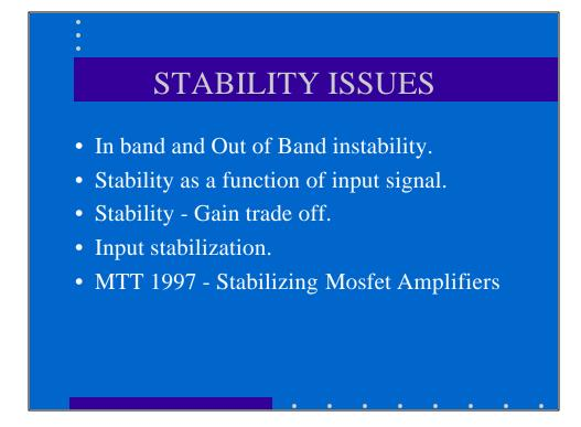
Vdmos instability is at lower frequencies and can be overcome with resistive loading of the gate circuit (1).
