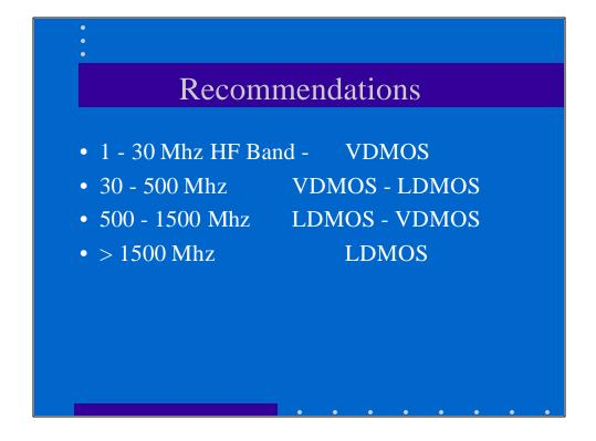
Polyfet has spent years developing both Vdmos and Ldmos devices. If we separate operating bands into HF, VHF and UHF, we can generalize on the type of technology which offers the best compromise between performance and reliability.
